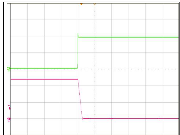
Figure 4: AVD50B-48S12 Output Voltage Shut Down By Remote Off V_{IN} = 48Vdc, I_O = I_{O,max}, 10mS/div
