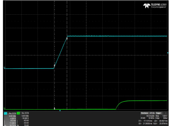
Figure 8: DS1600SPE-3 Output Voltage Startup Characteristic Vin = 180Vac Load: I_O = 129.8A I_{SB} = 3.5A Ch 3: V_O Ch 4: Pwr_GOOD
