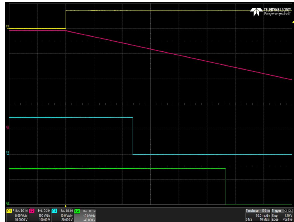
Figure 8: AIQ00ZPFC-01NL Turn-off Characteristic via PF Enable Vin = 115Vac/800Hz Load: Io = 0.19A Vo = 390V Cout = 2*150uF/450V Ch 1: PF ENABLE Ch 2: Vo CH 3: PFW Ch 4: LD_EN
