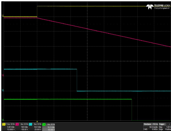
Figure 7: AIQ00ZPFC-01NL Turn-off Characteristic via PF Enable Vin = 115Vac/400Hz Load: Io = 0.19A Vo = 390V Cout = 2*150uF/450V Ch 1: PF ENABLE Ch 2: Vo CH 3: PFW Ch 4: LD_EN
