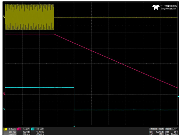
Figure 6: AIQ00ZPFC-01NL Turn-off Characteristic Vin = 115Vac/800Hz/0° Load: i_o = 0.19A Co = 2*150uF/450V Ch 1: Vin Ch 2: Vo Ch 3: PFV
