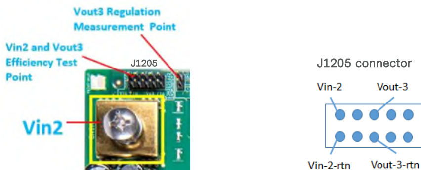
Figure 14 - Voltage sense locations for Vin2 and Vout3
